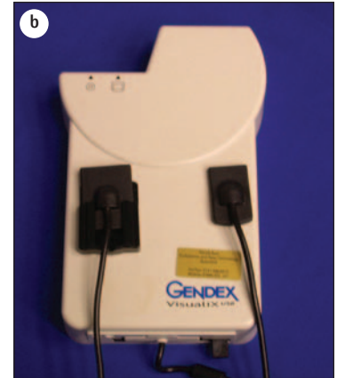
Fig. 8 An illustration of the computer screen produced by digital radiography, enabling immediate viewing and manipulation of the image. The sensor plate or 'film' may be either loose, resembling a conventional periapical radiographic film, which must be inserted into the machine for processing, or linked by cable to the processor as in b).
