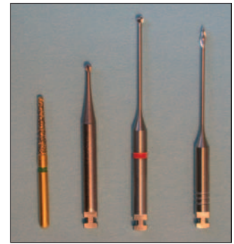
Fig. 14 Some of the burs specifically manufactured for endodontic treatment; a safe-tipped access bur; a long-shanked round bur; a swan-necked bur; a Gates-Glidden bur.
