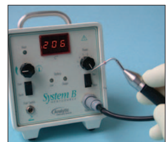
Fig. 11 The System-B heat source. When the ring on the handpiece is pressed as shown the tip of the plugger is immediately heated to the temperature selected.
