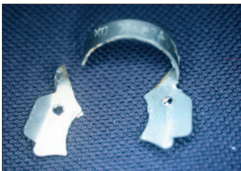
Fig. 8 Rubber dam clamps should always be protected with a length of dental floss in case they either fracture, as shown here, or are dropped in an unprotected mouth.
